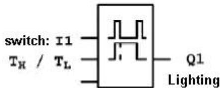
When the input "I1" has a pulse, the output "Q1" will be on and not off until the period "TH" be over. Keep the momentary switch holding down in period "TL", the light will be on all the time.
