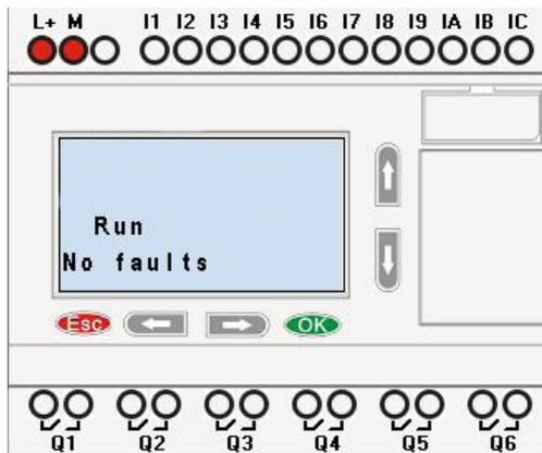
After pressing ESC key, FLC would be switched to function page and meanwhile open function menu as figure below shows.
