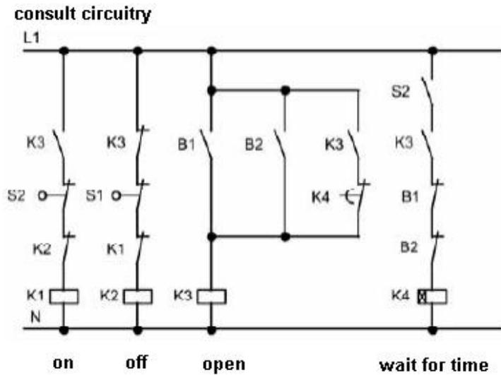
As long as the detector B1 or B2 detects someone approach, the switch K3 will be on and open the door.
