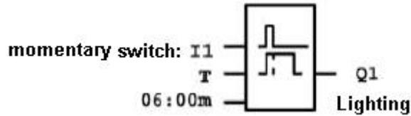
If input "I1" has a pulse, the output Q1 will be on and keep 6 minutes, then be off.
