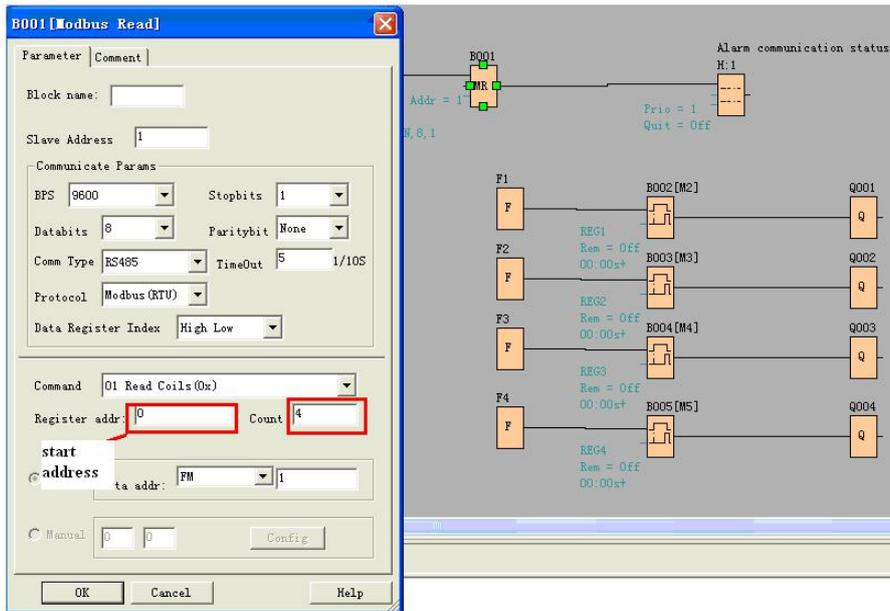
F is bit type flag. It can be used to receive bit data from slave device.
