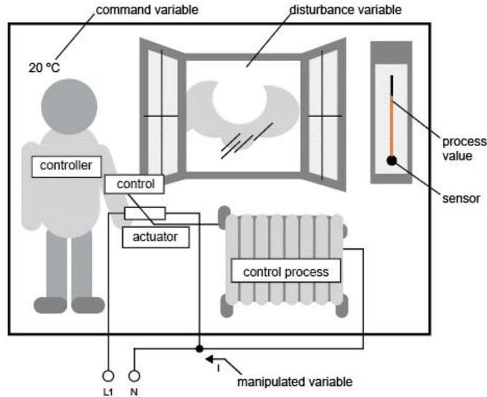
The control device is formed from the actuator and the control.
