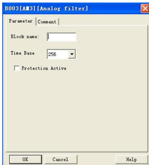
After you set the parameter, the analog filter calculates the average value of the samples and assigns this value to AQ.
