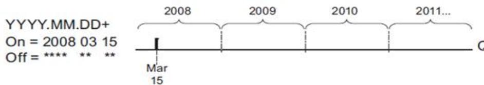
**Example 7:** Yearly mode on, Monthly mode off, Pulse off, On Time = 2008-12-15, Off Time = 2010-01-07: On December 15 of 2008 and 2009, the timer output switches on and remains on until January 7 of the following year. When the timer output turns off on January 7, 2010 it does NOT turn on again the following December 15.
