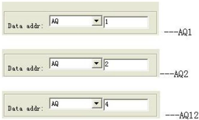
The number setting of Q, I, AQ are continuous. AQ12 cannot be set as AQ12 and should be set AQ4 as above figure shows.
