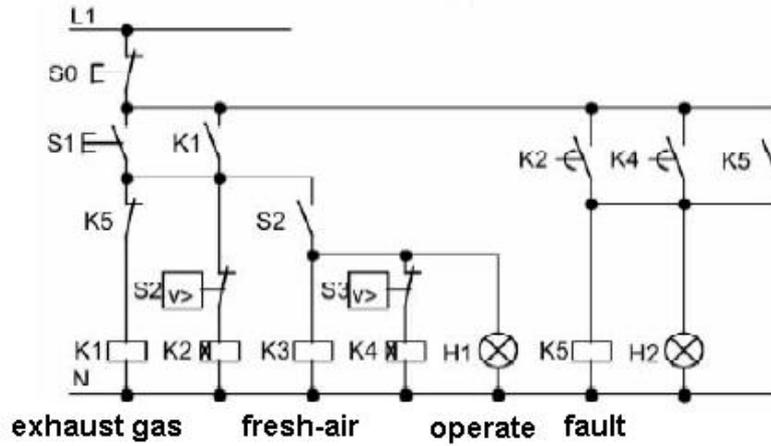
The fans are monitored by means of flow sensors. If no air flow is registered after a short delay time has expired, the system is switched off and an error message is generated, which can be acknowledged by pressing the off button.
