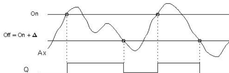
**Timing diagram B: Function with positive difference Delta**
