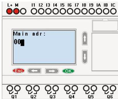
Change the address with arrow keys, and confirm with "Ok".
