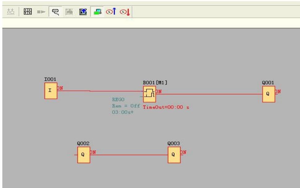
Under monitor mode, user can change the spare output (the input pin of Q is not connected to other blocks) state via FLC Logic Soft.
