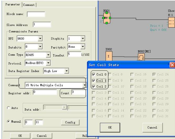
The above configuration is to force Q1, Q2, Q3 of Slave No.1 ON. " Coil 0" means pre-set the BIT 1 and " Coil 0" means pre-set the BIT 0 "Coil 0" is corresponding to the start address, Here is Q1.
