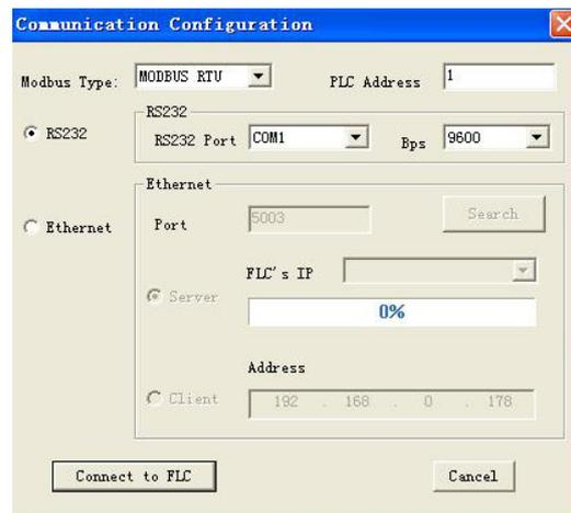
Fig. 7.10.10 Set Up Port and Baud Rate
