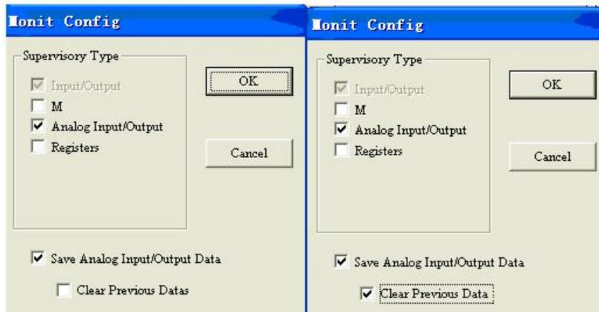
**Caution:** If the "clear previous data" is selected as well, then the history data cannot be saved, and then only the current monitor data can be saved, furthermore, the history data (previous monitor data) would be simultaneously cleared.
