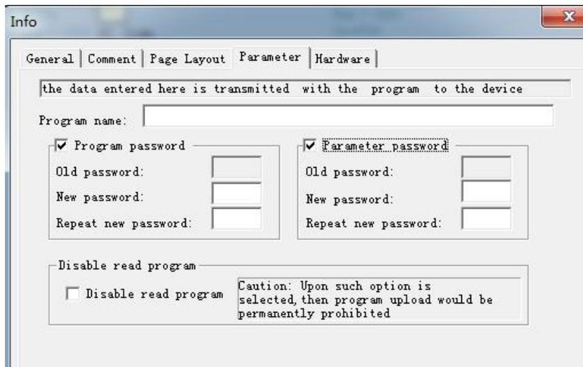
There are 2 password settings can be applied to the program, one is the program password, one is parameter password.
