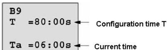
You are allowed to modify configuration time. Switch on/off time for a time segment.
