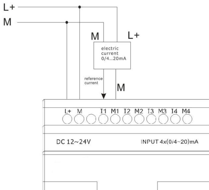
The above figure shows how to make a four-wire current measurement.
