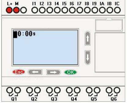
D. Modify value by pressing arrow keys and confirm with OK key.
