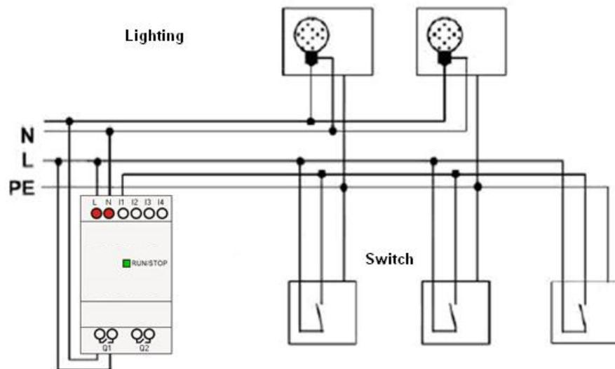
The wiring of a lighting system with FLC is the same as standard corridor or stairway lighting systems. Only the automatic lighting timer/pulse relay is replaced. FLC lets you quickly and easily combine all those functions in a single dual-function switch SFB, without additional wiring and expenditure.
