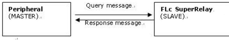
However, the “Modbus Read” or “Modbus Write”(next chapter will introduce it) function block would be utilized if FLC shall be required to play a role of master to communicate with other devices. As the following figure shows:
