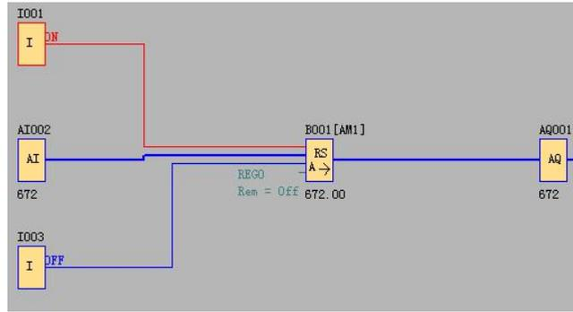
When the I3 turns to HIGH, the value of this function block will be reset to 0.
