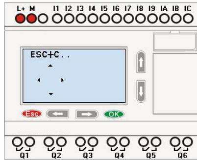
Cursor keys can be controlled in this page by press arrow keys and ESC key at the same time. If FLC has several alarm interfaces in the same period and it only displays the message with highest priority in the function block, also you may go through all alarm messages by pressing ▲ or ▼ key.
