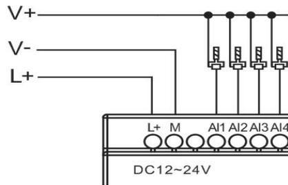
**\* Analog inputs current Inputs (0...20mA)**
