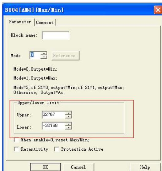
In the dialog box of Max/Min block, there is a upper/lower limit setting, when the block output the AQ value is less than the lower value, the AQ shall be equal to the Lower value; While the block output the
