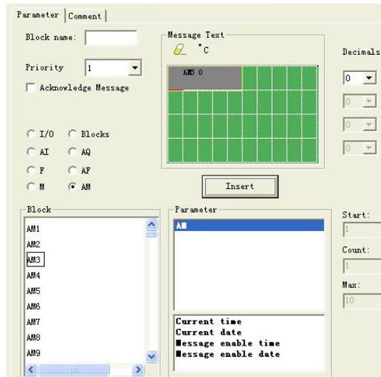
With text message, the text can display big number (6 bits or 4 bits). (This feature only can be used in FLC-12 CPU).
