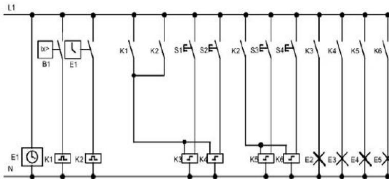
Lighting lamp can be operated by pulse relay controlled by button besides the door. Pulse relay can be repositioned by means of timer and lightness sensitivity switch. Pulse relay may shorten pulse width of "off command".
