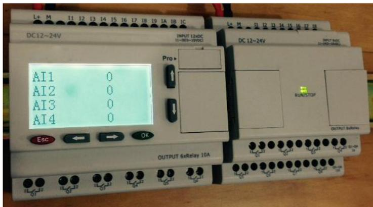
**Note:** If you need install the expansion and CPU on different rows, you need order the longer flat connection which is used to connected with CPU, the longest distance can be 200 meters between the CPU and the end expansion module.
