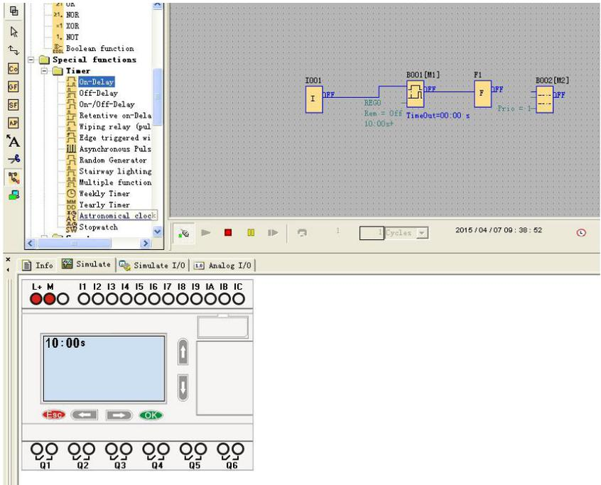
C. Press "ok" for 3 seconds and enter into edit mode.
