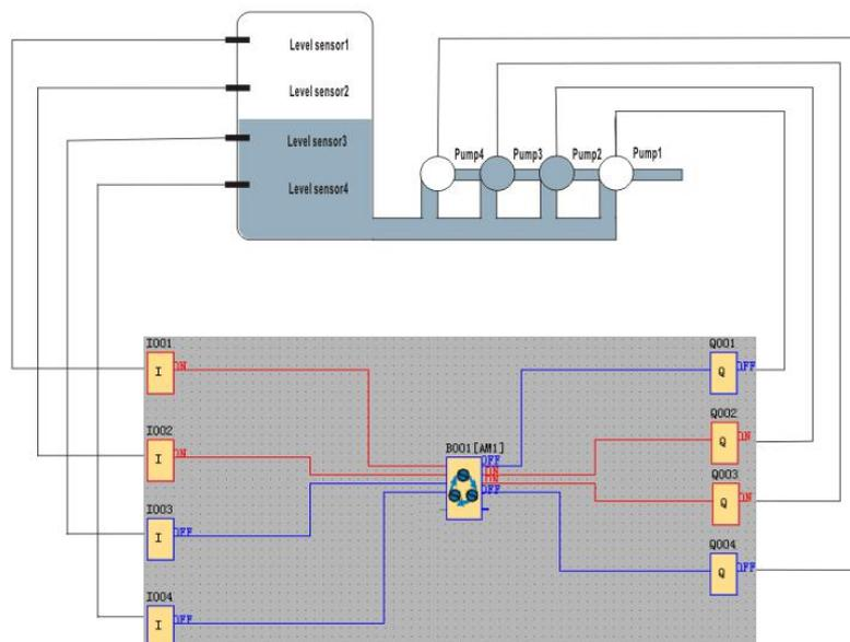
The "number of outputs controlled" parameter is fixed at 4.
