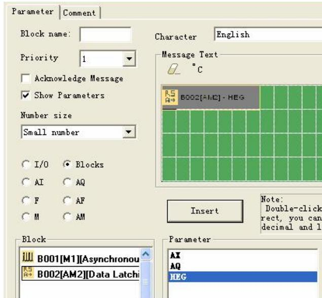
There is Modbus address for the HEG, so you can also can change the HEG value by Master (Touch screen etc.). You can found the address in the modbus RTU protocol (Memory map) file.
