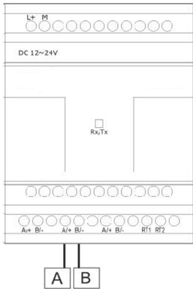
If "RT1", RT2" terminal are short connected, one 120R resistor will be connected between A/+ and B/-
