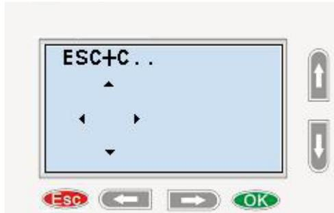
Switch the screen to current page(above shows) by pressing the Left or Right key, and press ESC key and arrow keys at the same time, then the corresponding cursor keys will turn on and give off a high trigger!
