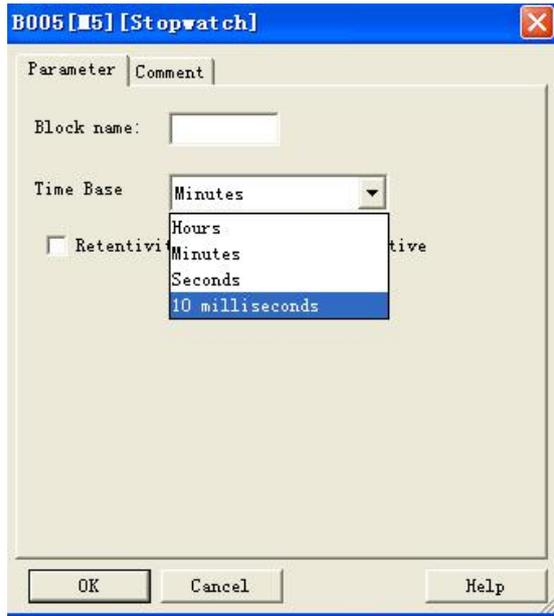
The time base for the elapsed time can be in hours, minutes, seconds, or 1/100ths of seconds (units of 10 milliseconds). The smallest time base, and therefore the resolution, is 10 milliseconds, or 1/100ths of seconds.
