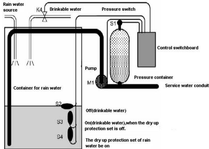
The rain water is collected in the container and then pumped to service water ductwork through pumping station. So you can apply rain water as drinkable water. If the rain water in the container dried up, this system can supply drinkable water.
