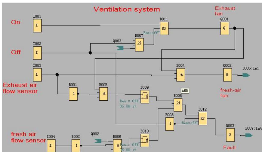
You can invert output Q3 to use output messages at Q4. Relay Q4 only drops out if main power is lost or if there is a fault in the system. The output can then be used for a remote message.
