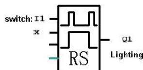
When the input "I1" has a pulse, the output "Q1" will be on or off.
